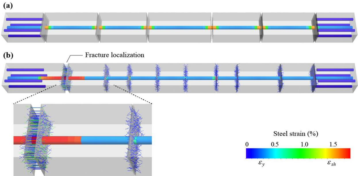
**Fig. 4** Simulated crack patterns and fibers that bridge crack faces at 0.57% strain: (a)  $V_f=0$ ; (b)  $V_f=0.5\%$
