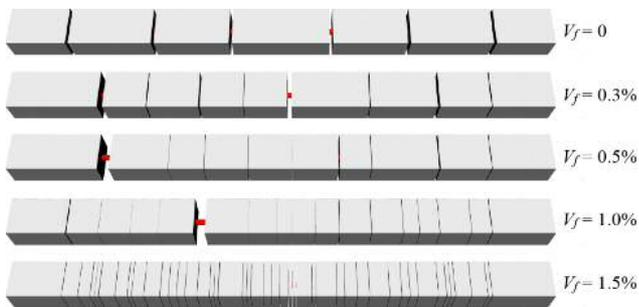
**Fig. 5** Simulated crack patterns at 1.2% strain
