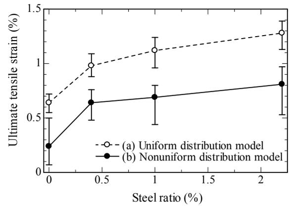
**Fig. 9** Ultimate tensile strain as a function of steel ratio
