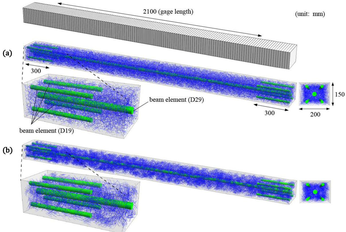
**Fig. 1** Discretized cement matrix, steel bars, and fibers ( $V_f=0.5\%$ ): **(a)** uniform distribution model; **(b)** nonuniform distribution model
