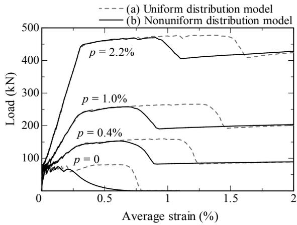
**Fig. 8** Tensile load-average strain curves ( $V_f=1.5\%$ )
