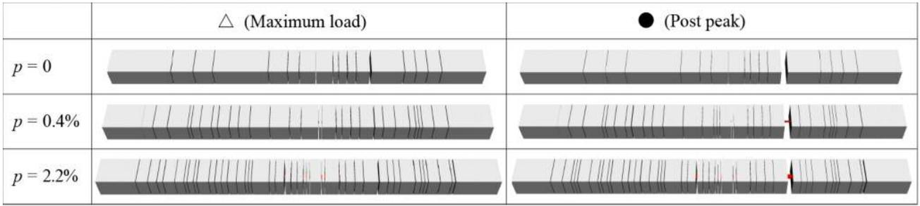
**Fig. 7** Simulated crack patterns ( $V_f=1.5\%$  - uniform distribution model)
