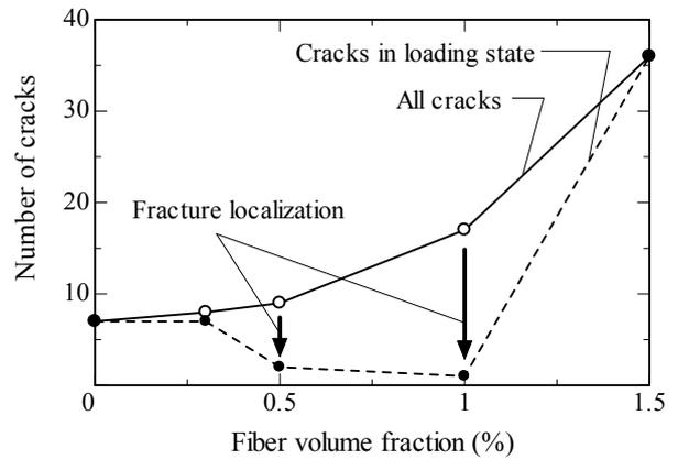
**Fig. 6** Number of cracks as a function of fiber volume fraction at 1.2% strain
